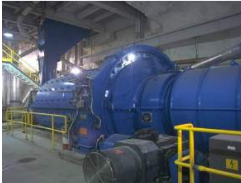
A semi-autogeneous grinding mill underground (TRL = 9)
