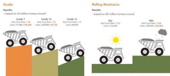
Figure 11: Comparing rolling resistance using the Leighton Contractors Best Truck Ratio
